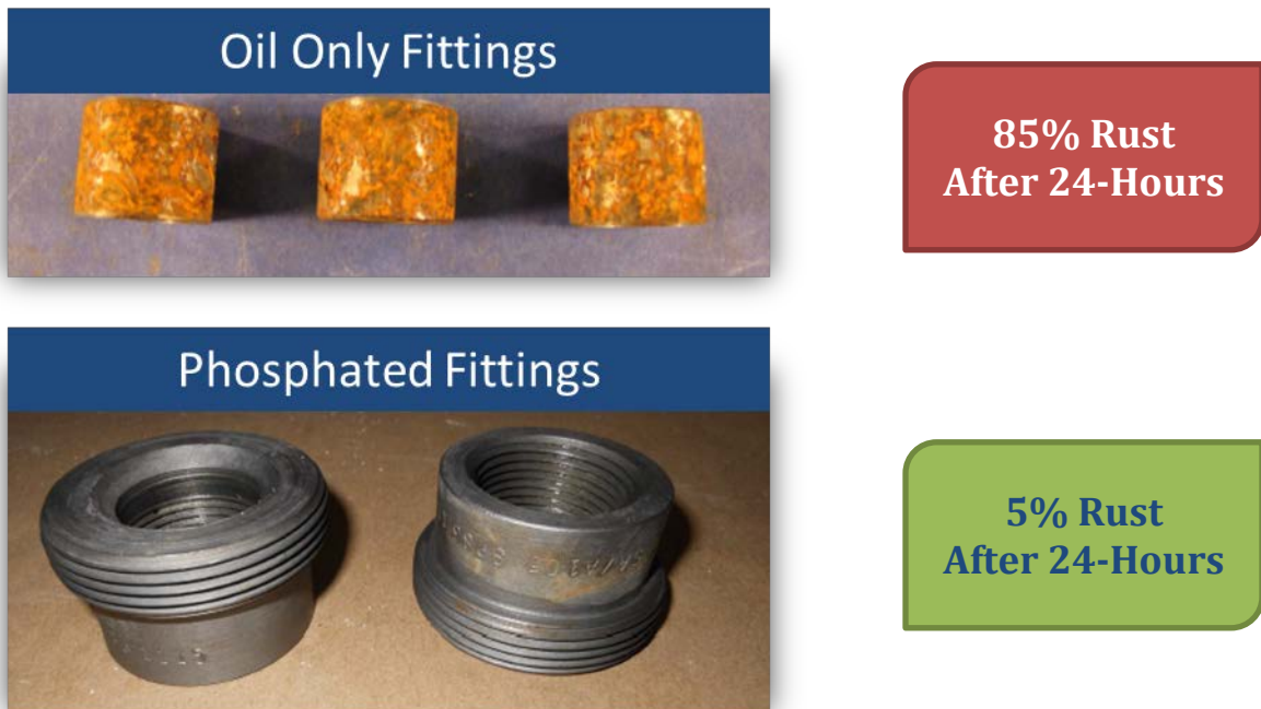
Figure 3: Oil-Coated and Phosphate-Coated Fittings After 24-Hour Salt Fog Test
