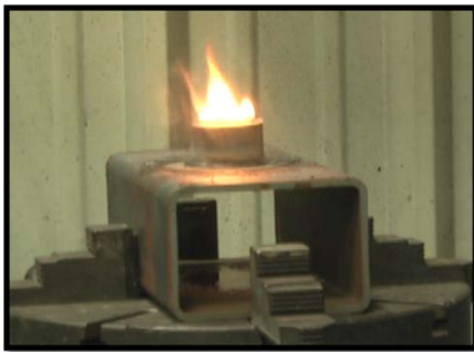
Figure 1: Flame After Welding Oil Coated Fitting
