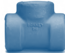
Tee Threaded Class 2000 - 1/4" to 4" Class 3000 - 1/8" to 4" Class 6000 - 1/8" to 4" Socket Weld Class 3000 - 1/8" to 4" Class 6000 - 1/8" to 4" Class 9000 - 1/2" to 2"
